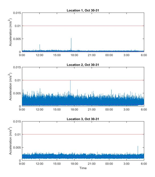
Figure 1: RMS particle accelerations at Location 1, 2 and 3 on October 30-31, 2017. The magenta dash line represents the mean baseline RMS particle acceleration calculated from October 5 to 16 at each location. The red line shows the 0.01 m/s<sup>2</sup> threshold of the RMS particle acceleration.
